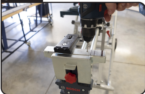
PRE-DRILL HOLES FOR ADAPTER BLOCK
