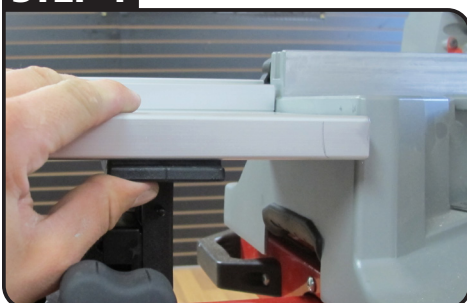
SOME SAWS HAVE HIGHER DECKS REQUIRING SPACERS FOR PRECISION ADJUSTMENT BLOCKS
